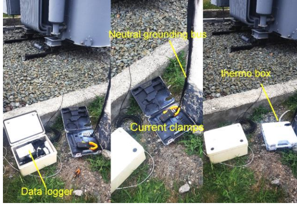
Figure 4. Current sensor on the grounding bus of the 2.5 MVA power transformer at the Ininskaya power substation
