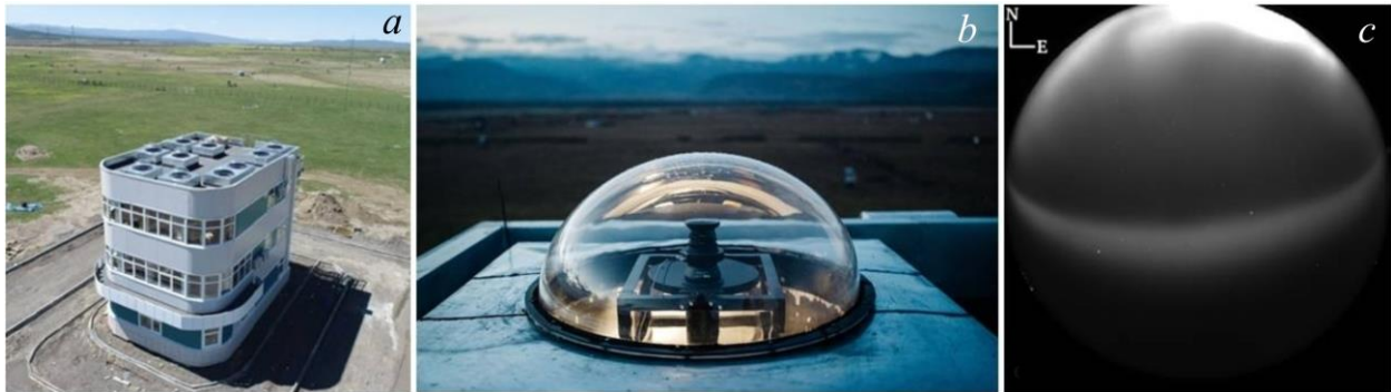
Figure 17. NHC RAS: Complex of passive optical instruments at GPO ISTP RAS. Building (a); an all-sky camera in the dome space (b); SAR-arcs detected with the all-sky camera at a wavelength of 630 nm during the April 23, 2023 strong geomagnetic storm (c)
