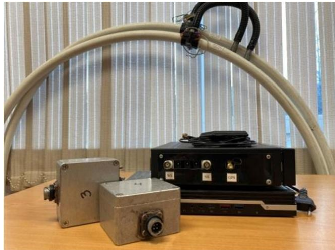
Figure 1. Schematic diagram of the lightning location network's recorder ( a ); a set of equipment for one of the stations ( b )
